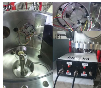
Figure 30: a) the beam chopper mounted in the RBS-C chamber, b) the electronic controller box of chopper.
